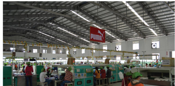
Transparent roof panels and more windows maximize use of day light
