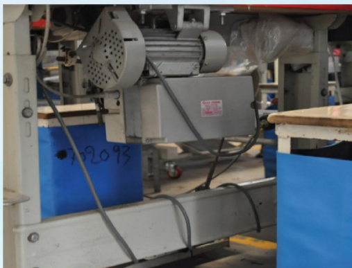
Almost sewing machines were upgraded to servo motors
