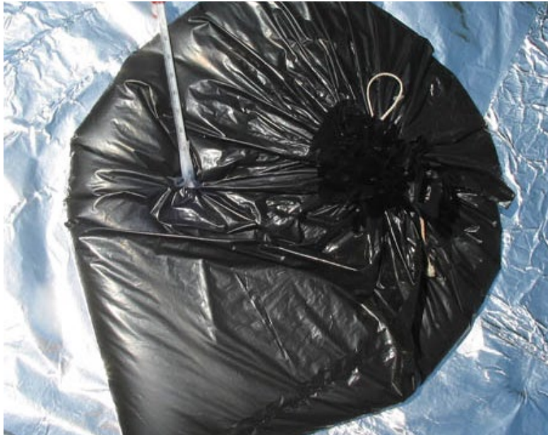
Figure 1. This image shows an example of a black bag batch solar collector sitting on top of a foil-covered Styrofoam panel.
